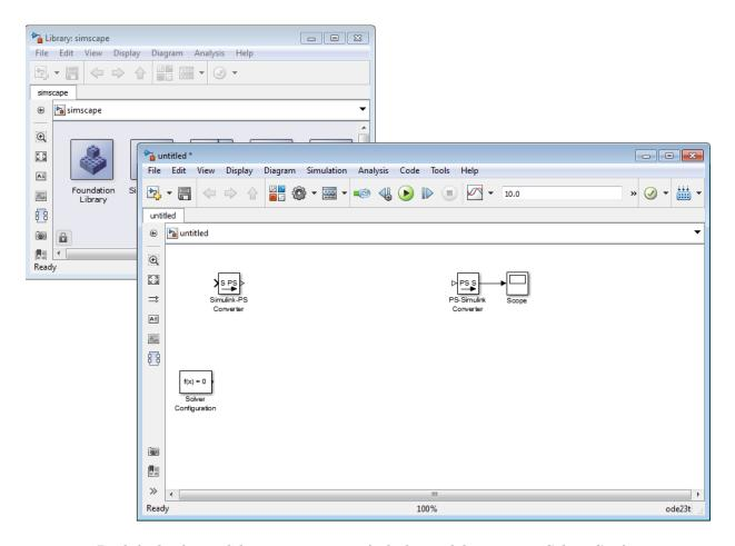
By default, the model name is not specified, the model contains a Solver Configuration block with the default solver set to ode23t, a Simulink-PS Converter block, and a PS-Simulink Converter block connected to a Scope block.
