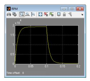
For the first 0.1 seconds, the motor has no external load, and the speed builds up to the no-load value. Then at 0.1 seconds, the stall torque is applied as a load to the motor shaft. Zooming in on the RPM and Motor Current scopes shows that the model matches the manufacturer parameters for no-load speed, no-load current, and stall torque.
