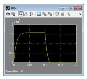
**3** Try varying the load torque to find the maximum torque at this reduced voltage. Double-click the Step source block, enter different final values for the input signal, and rerun the simulation.
